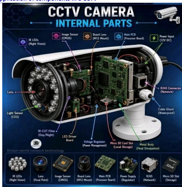
Exhibit 2: Application of components in a CCTV
